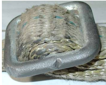
EXCESSIVE WEAR OF HARDWARE OR CRACK (Cracks are indicated by fine black lines)
