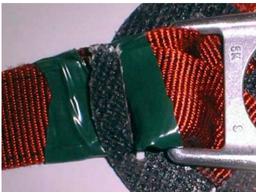
UNAUTHORIZED REPAIR / ALTERATION
