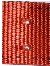
HOLES IN WEBBING
