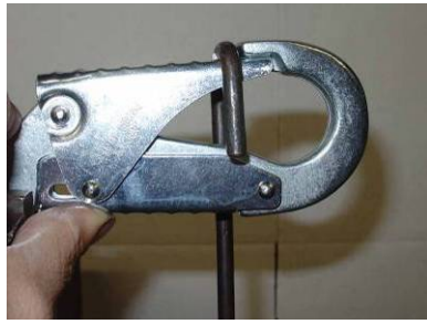
KEEPER TENSION: Less Than 2.5 lbs *Note: Locking Mechanism must be depressed for Keeper Tension check.
