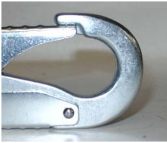
DEPTH OF KEEPER IN BILL 3/16" Minimum
