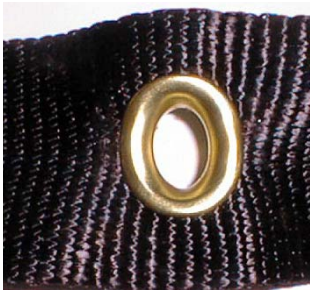
BENT OR DEFORMED GROMMETS
