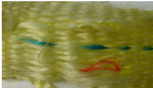
EXCESSIVE WEAR EXPOSING RED WEAR MARKER (1" YELLOW WEB)
