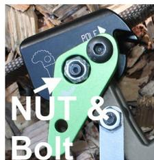
**Serrated Rotosnap (locator rib) Fig. 3c**
