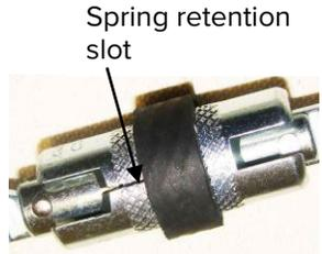
2. The cams of the WebGrab and BuckGrab rotate freely and lock on the strap / rope when properly adjusted on the pole and the user's weight is on the unit.
