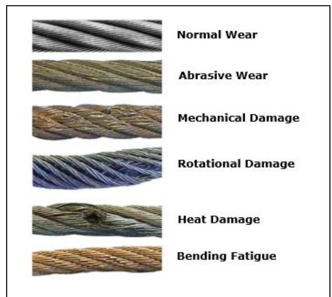
Figure 7: Examples of equipment damage
