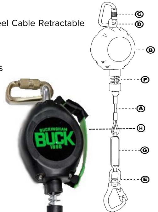
Figure 1a: Key components of Class 2 Self-Retracting Devices
