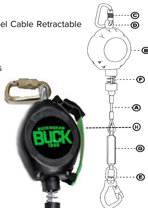
Figure 1a: Key components of Class 2 Self-Retracting Devices
