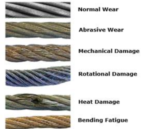
Examples of Cable Damage
