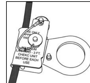
6. Check locking action by pulling down on rope grab handle.
