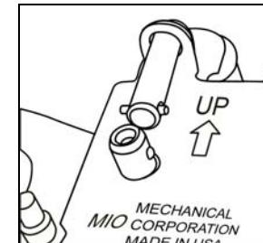
5. Make sure that locking pin balls appear on outside of main assembly and the direction arrow on the housing is pointing up.
