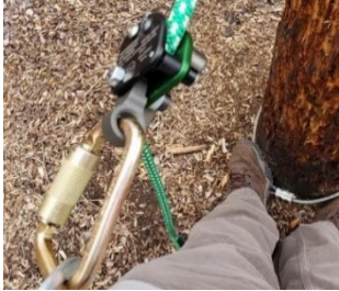
LeverGrab positioned on left side with Carabiner oriented as it leaves the factory (Right hand adjustment set-up).
