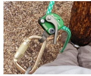
LeverGrab positioned on left side with Carabiner reversed (Left hand adjustment set-up)
