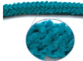
Rope with Excessive Abrasion Wear
