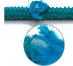
Rope with Broken or Cut Strands
