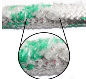
Rope with Excessive Abrasion Wear
