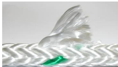
Rope with Broken or Cut Strand
