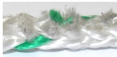
Rope with Excessive Abrasion / Wear
