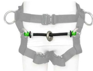
The rings have an approximate inside diameter of 1 5/32" (29mm) for the small ring (PN 100A), 1 7/8" (48 mm) for the large ring (PN 200A) and 2 1/2" (63.5 mm) for the extra-large ring (PN 300A). All three rings have a Minimum Breaking Strength (MBS) of 5000 lbf. (23 kN) in all directions.
