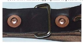
13) Fold the Foot Strap over the Split Ring so holes #1 & #2 fit onto the Rivets in holes #3 & #4
