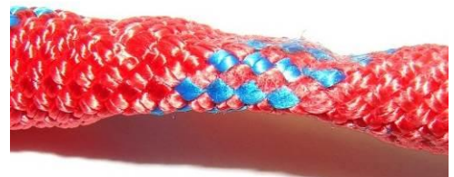
Inconsistent Diameter / Compacted Area
