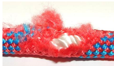
Excessive Abrasion / Wear - Contrasting Core visible
