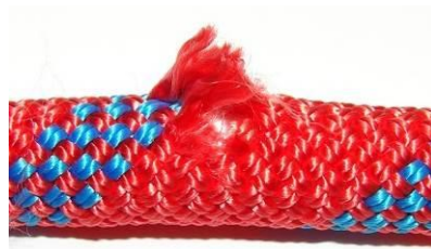
Broken or Cut Strands
