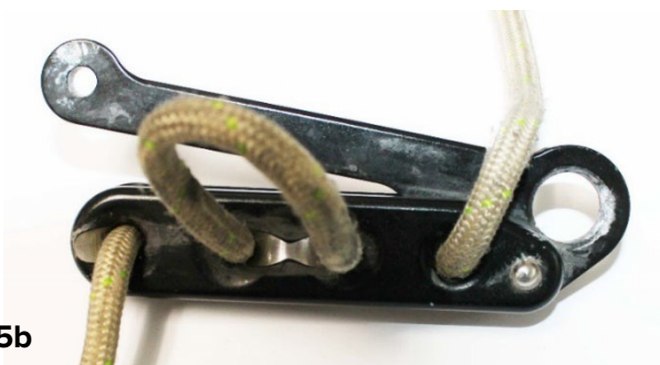
CORRODED DESCENDER WITH EXCESIVE WEAR GROOVES / MARKS FROM DESCENT LINE FRICTION
