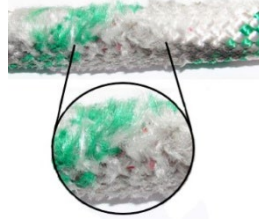
Rope with Excessive Abrasion Wear
