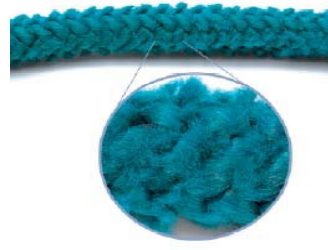
Rope with Excessive Abrasion Wear
