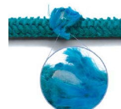
Rope with Broken or Cut Strands
