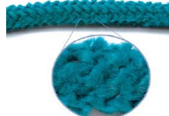
Rope with Excessive Abrasion Wear
