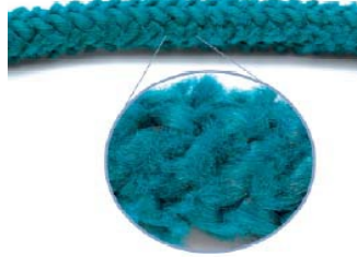
Rope with Excessive Abrasion Wear
