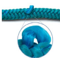
Rope with a Pulled Strand
