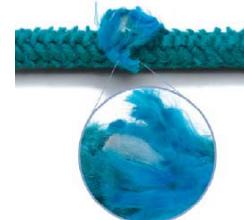
Rope with Broken or Cut Strands
