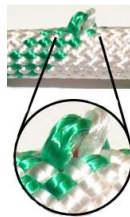
Rope with a Pulled Strand
