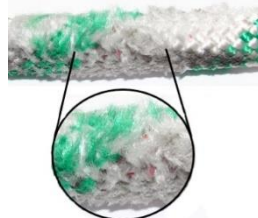
Rope with Excessive Abrasion Wear
