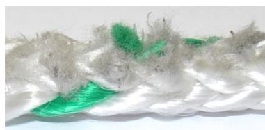
Rope with Excessive Abrasion / Wear
