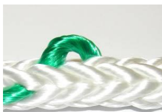
Rope with a Pulled Strand
