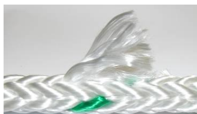
Rope with Broken or Cut Strand
