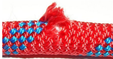
Broken or Cut Strands
