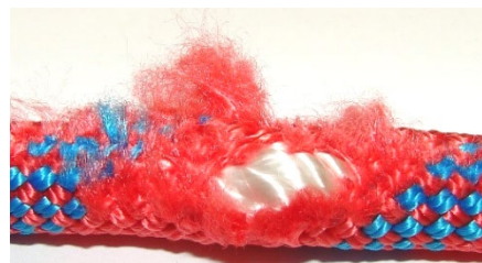
Excessive Abrasion / Wear Contrasting Core visible
