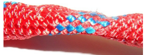
Inconsistent Diameter / Compacted Area
