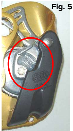
a. Depress silver button on side of locking wheel
