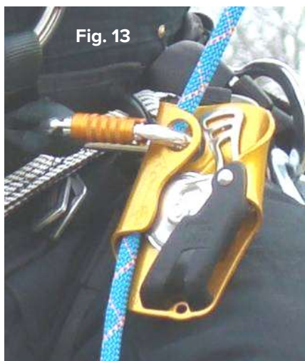
c. Attach carabiner to Fall Arrester
